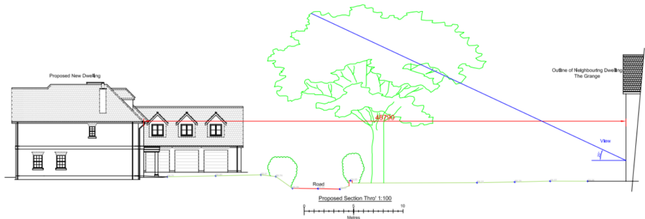
Site Section on the east elevation showing the proposal's relationship with the Grange (some 48.7m to the east on the other side of Ashton Road) including the 25-degree rule
